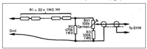
Third, if these resistors run too close to their maximum rated power dissipation they will change in value and affect the meter reading, so the whole resistor chain must be substantially over-rated.
